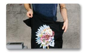
Cure: The final step in the process is to use a heat press or tunnel dryer to cure the ink into the garment. Heat curing ensures ink longevity so your finished prints will be colourfast, machine-washable, soft to the touch, and stretch without cracking.
